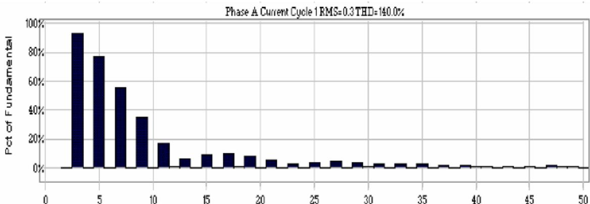
Harmonic voltages and currents are integer multiples of the fundamental frequency. On 60 Hz supplies, for instance, the 5<sup>th</sup> harmonic is 300 Hz; the 7<sup>th</sup> harmonic is 420 Hz, and so forth. When all harmonic voltages and currents are added to the fundamental, a waveform known as a “complex wave” is formed. An example of complex wave consisting of the fundamental (1<sup>st</sup> harmonic) and 3<sup>rd</sup> harmonic is illustrated in Section 2, Figure 8.
