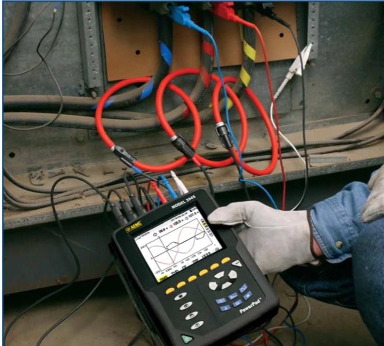
In addition to the full range of harmonic measurements, the AEMC 3945 can measure and record short-term flicker, capture up to 50 transients or other disturbances to 1/256<sup>th</sup> of a cycle, record voltage and current unbalance, trend recordings and monitoring of a number of parameters based on min/max limits and “photograph” up to twelve data displays. Comprehensive software is provided to assist in report compilation.
