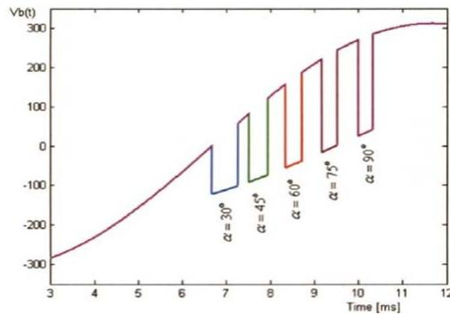
Fig 32 : Notch depth variations on firing angle changes
