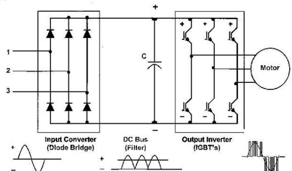
Fig 4 : Simplified 6 pulse AC VFD schematic
