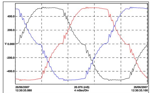
Fig 3 : Example of line voltages distorted by AC VFDs (8.8% U<sub>thd</sub>) .
