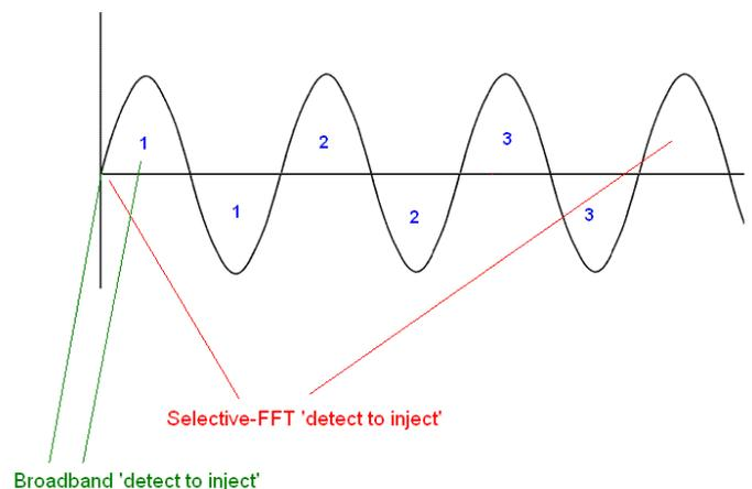
Fig 23 : Comparison of 'broadband' and 'selective FFT' active filter response times
