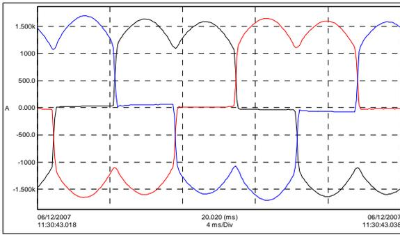
Fig 9 – Example of DC SCR drive at moderate load (31.51% Ithd)
