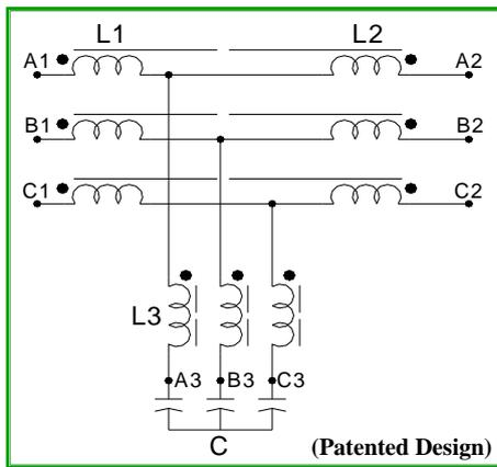
Fig 13 – Advanced wide spectrum filter schematic.
