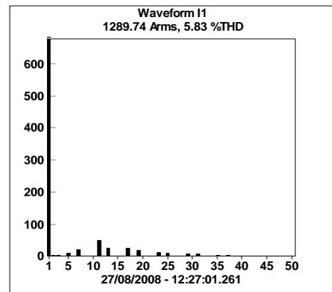
Fig 17 – 900HP/630kW DC SCR drive harmonic current spectrum (I1) in AMPS. With T type wide spectrum filter - 5.83% Ithd
